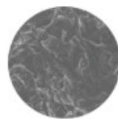
Surface areas are increased through blasting by highly biocompatible Calcium Phosphate Media.
